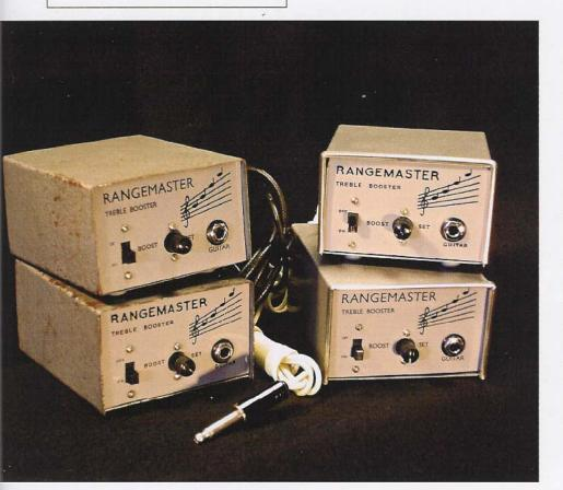
A note picked hard will sound only a bit louder than one picked softly, but what we are ultimately looking for is a different tone or timbre when picked at different hardnesses. The Rangemaster, in its original form, has this quality. It is extremely responsive, as are most of the older based clones. Some of the newer ones I tested were less so-so, but they perform admirably.
